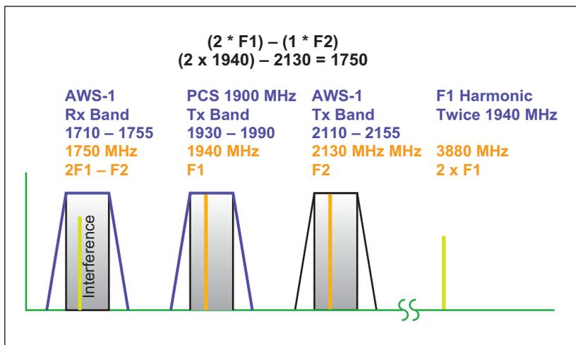
Figure 3. PIM causing receiver de-sense at 1710 MHz.
