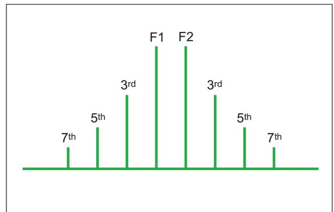
Figure 1. Carriers F1 and F2 with 3<sup>rd</sup> through 7<sup>th</sup> order products.
