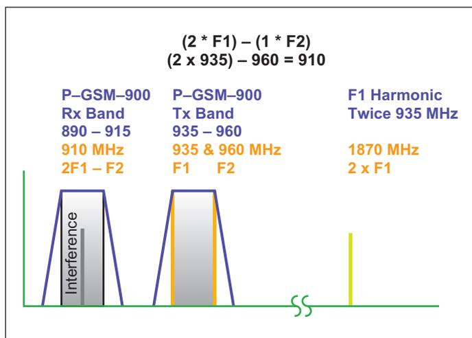
Figure 4. PIM causing receiver de-sense at 910 MHz.
