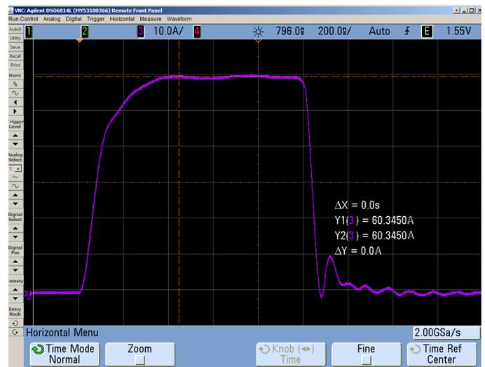
Typical 800ns Output Waveform, 60A
